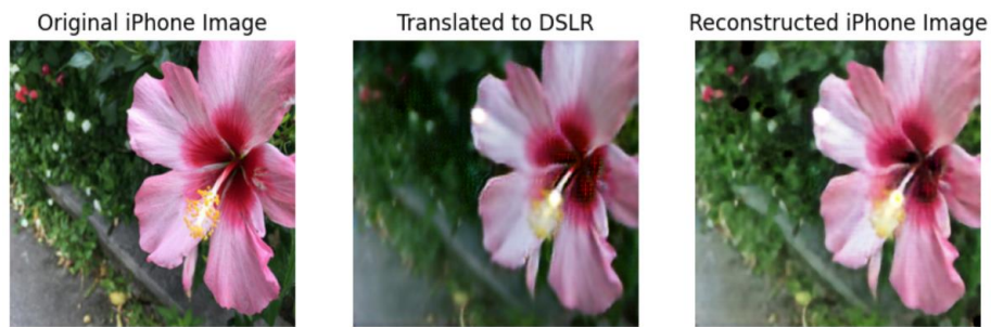
Figure 7: An iPhone image from the 'testA' dataset was fed into generator G to produce a translated DSLR image. This generated DSLR image was then passed through generator F to reconstruct it back to the original iPhone image. Time taken for translation to DSLR was 0.09126 seconds.
